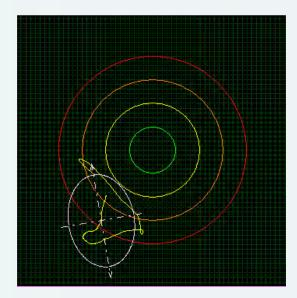
It is designed to quickly quantify the subject's ability to minimize and control his/her sway as well as the symmetry of weight-bearing.
